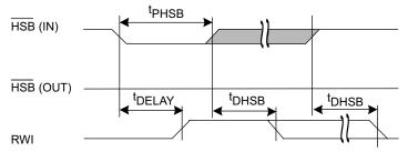
$\overline{\text{HSB}}$  pin is driven high to V<sub>CC</sub> only by Internal 100K $\Omega$  resistor, HSB driver is disabled SRAM is disabled as long as HSB (IN) is driven LOW.
